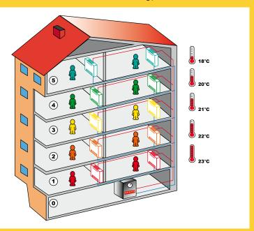
Balancing also plays an important role in distributing water supply, allowing all housing units to obtain the same amount of water, even when multiple people are using water simultaneously.
